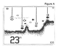
The range of the graphic display is shown to the right of the graphic information. The upper number is 0 indicating the surface of the water, the lower number is one of the 9 ranges available which best matches the depth of the water. As the depth of the water changes, the range changes as necessary in order to retain a bottom representation on-screen.
